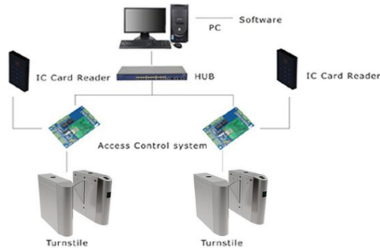
Access Control System
